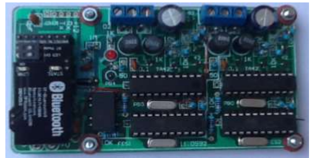
Figure 7. The proposed pulse generator circuit of FES
